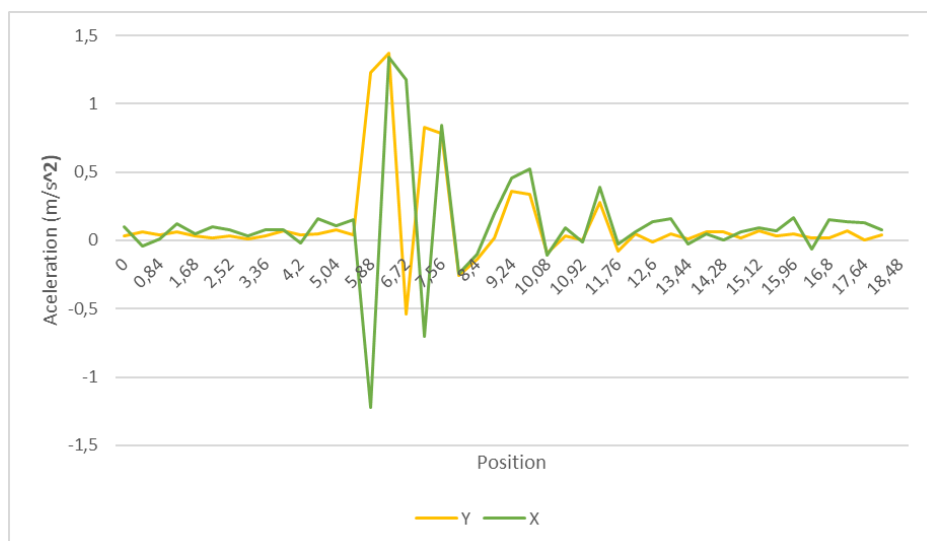
Graphic 2 - Acceleration measured on a section of the permanent way. Starting position: -15.832855135055894, -47.947129444860806 ; ending position: -15.832833846262513, -47.947298423969954; liquid cargo transported: 9,5 tons; velocity: 76 km/h.
