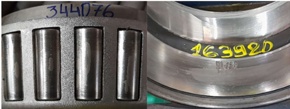
Figure 33: Micro spalling of the cone and cup (Source: MRS)
