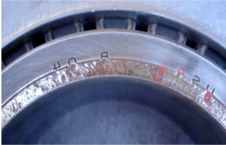
Figure 35: Face wear on the bearing cone, class K
