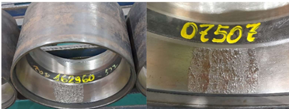
Figure 34: Severe cup spalling (Source: MRS)
