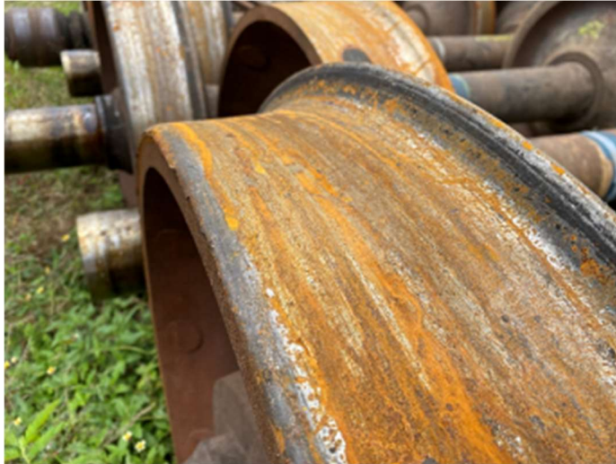
Figure 39: Excessive wheel wear (Source: MRS)
