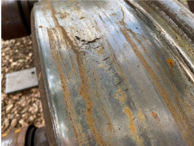
Figure 37: Contact Fatigue (RCF) (Source: MRS)
