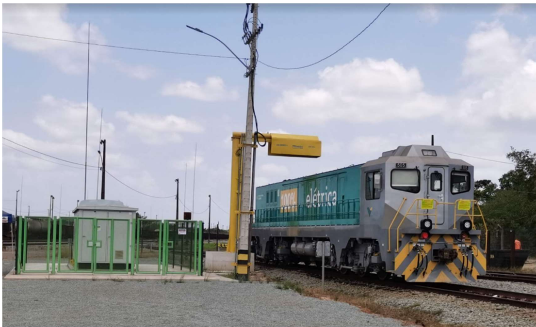
Figure 2.3 - CRRC BEL with battery charger and reverse pantograph for EFC (received in April 2022)
