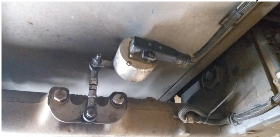
Figure 7 - Alstom Citadis 402 Tram Load Sensor – Rio de Janeiro Tramway VLT Carioca
