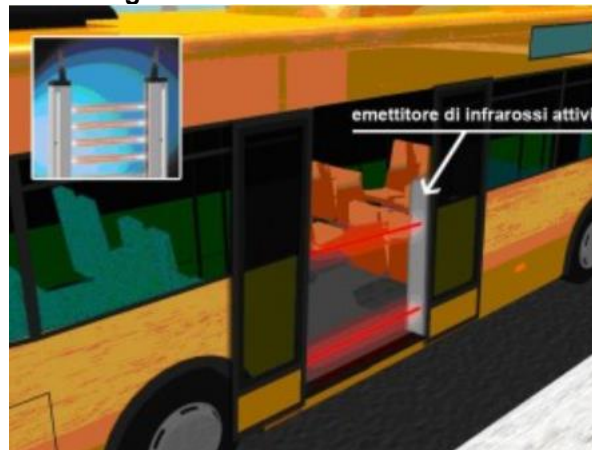
Figure 11 - IR Beam on bus door
