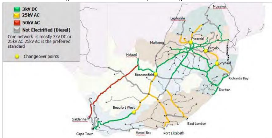
Figure 3 – South Africa's rail system voltage distribution
