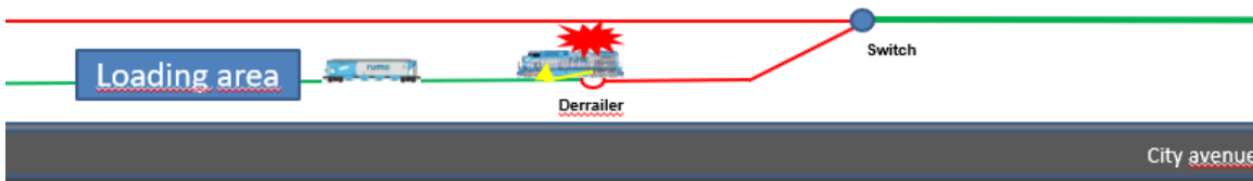
FIGURE 15 - DURING THE MANEUVER TO THE MAIN LINE THE LOCOMOTIVE DERAILS ONE WHEEL AT THE DAMAGED DERAILER
