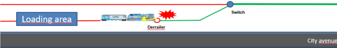
FIGURE 14 - COMPOSITION PASS THROUGH THE DERAILER ON THE WRONG POSITION, DAMAGING THE EQUIPMENT
