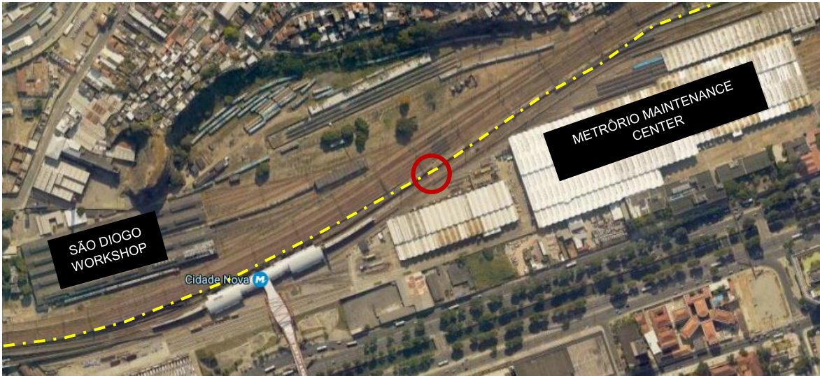
Figure 12 – Location of MetrôRio Maintenance Center and SuperVia's São Diogo Workshop, with special focus on the interconnection tracks between the systems (Source: Google Maps)
