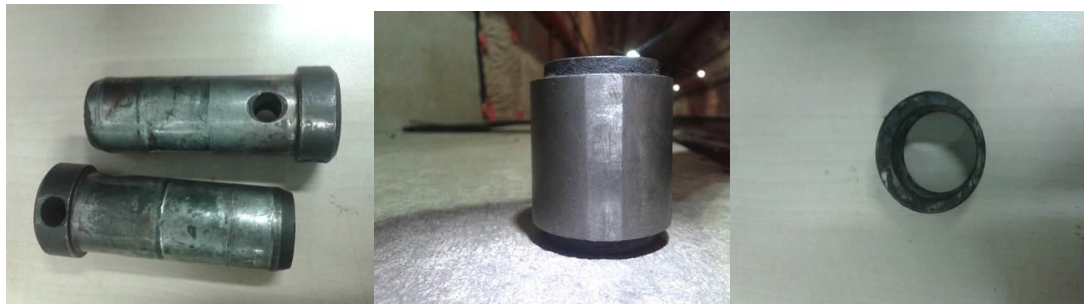
Fig 34: Point Machine Components Replaced
