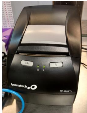
Figure 28 - DC 1000 and thermal printer used for selling and printing out the tickets with QR Code solution.
